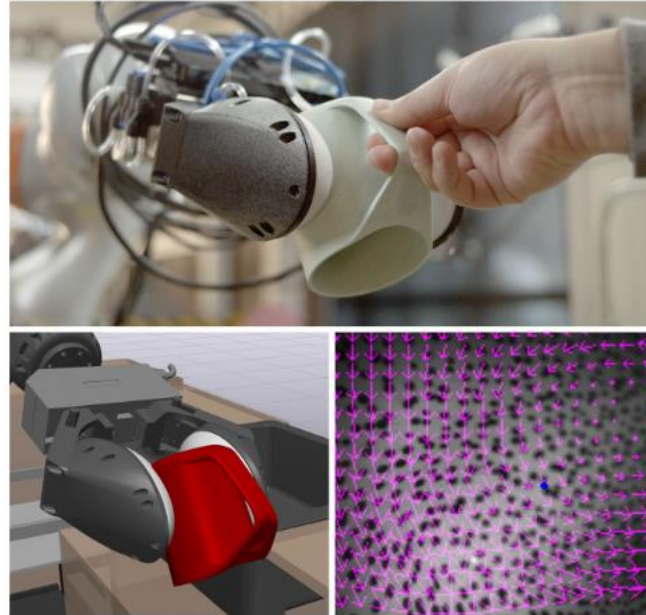
Fig. 1: Top: Highly compliant Soft-bubble parallel gripper of a robot arm grasping an object. Bottom-left: In-hand pose estimate during this interaction; Bottom-right: Shear-induced displacements tracked on the interior of this sensor.
