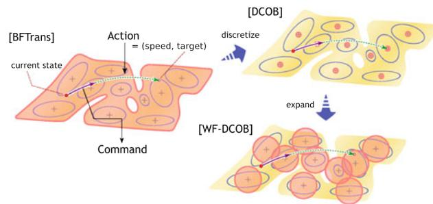
**Fig. 3** Relations of the proposed methods; BFTrans, DCOB, and WF-DCOB. BFTrans is an action converter from the agent's action into a command sequence for the robot. DCOB is a discrete action space obtained by discretizing the input space of BFTrans. WF-DCOB directly learns in BFTrans, but the actions are constrained around the actions in DCOB. Thus, WF-DCOB is regarded as an extension of DCOB.
