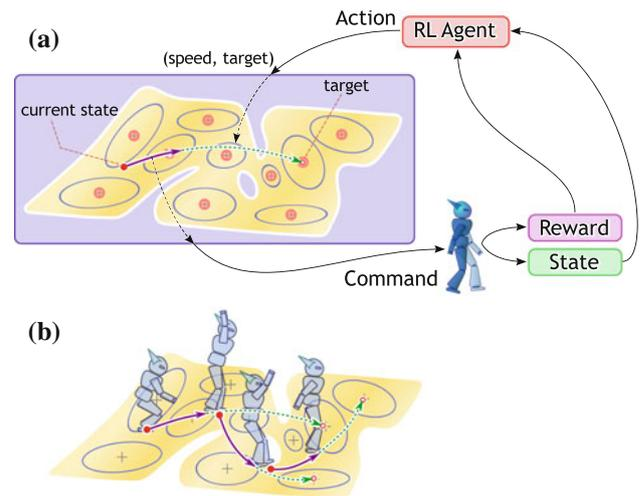
**Fig. 2** Overview of DCOB. **a** DCOB is a discrete action space generated from BFs. An action in DCOB selected by the RL agent is converted into a command sequence for the robot. **b** Acquired motion is generated by a sequence of the actions in DCOB
