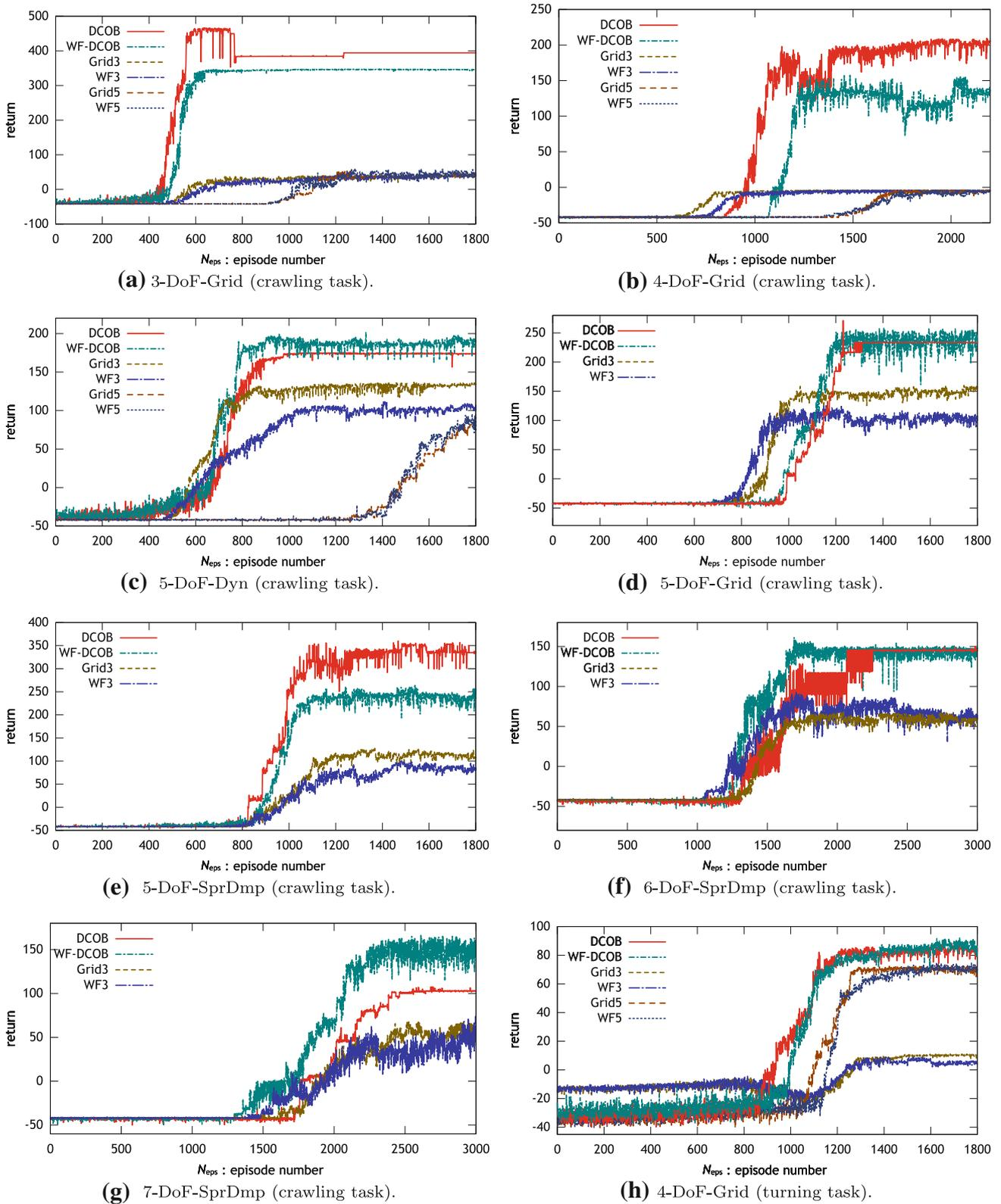
**Fig. 8** Resulting learning curves of the crawling task. In every graph, each curve shows the mean of the return over 15 runs per episode
