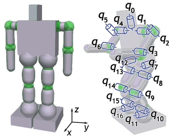
Fig. 6 Simulation model of the humanoid robot
