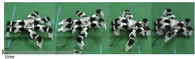
**Fig. 15** Snapshots of an acquired crawling motion of King Spider (4.8, 5.4, 6.0, 7.2 s)
