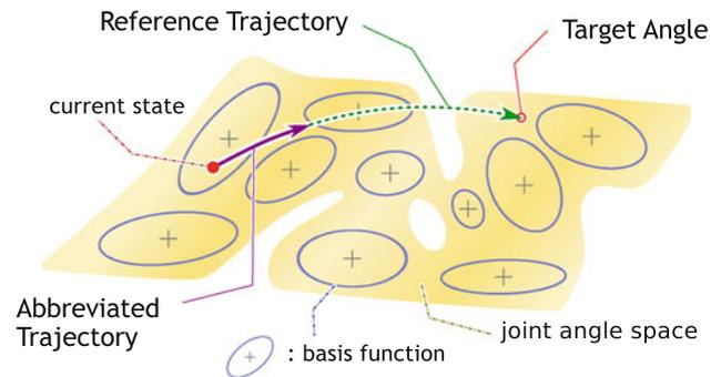
**Fig. 4** Illustration of how an action in the BFTrans is executed. First, a reference trajectory is generated, then it is abbreviated. The reference trajectory may change the state greatly, so the obtained motion is coarse. To make the motion fine, the trajectory is abbreviated
