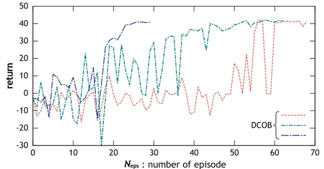
**Fig. 16** Resulting learning curves of the crawling task of Dinosaur. Each *curve* shows the return per episode in a run
