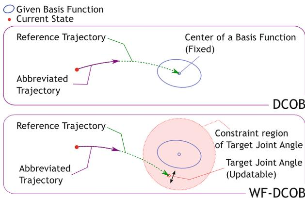
**Fig. 5** Illustration of the comparison of DCOB (*top*) and WF-DCOB (*bottom*). In both methods, the trajectory is calculated in the same manner as the BFTrans. The difference is that in DCOB, the target state is the fixed center of a selected BF, while in WF-DCOB, the target state can change but is constrained around a corresponding BF
