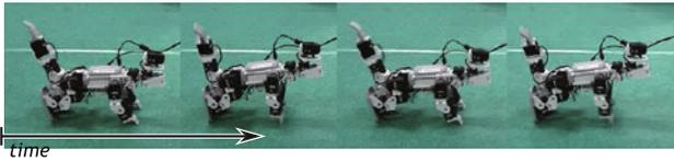
**Fig. 17** Snapshots of an acquired crawling motion of Dinosaur (7.2, 7.6, 8.0, 8.6 s)
