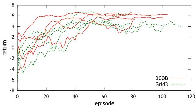
**Fig. 12** Resulting learning curves of the crawling task of King Spider (raw data). Each *curve* shows the return per episode in a run. To see the tendency of each curve, a low-pass filter with a time constant of ten episodes is applied
