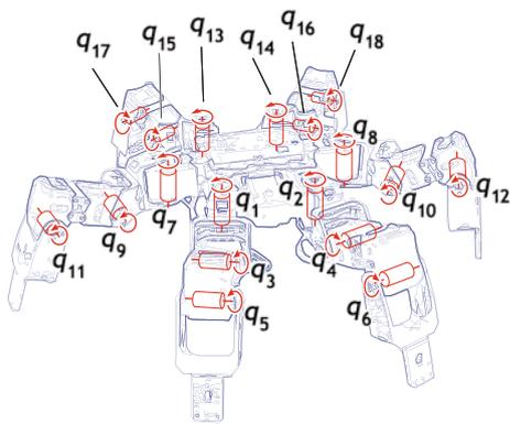
**Fig. 10** King Spider (ROBOTIS Bioloid) which has 18 DoF
