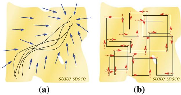
**Fig. 1** Illustration of a trajectory-wise exploration (a) and a graph search-like exploration (b) in the state space of a robot. In both figures, the *lines* denote the instances of the exploration trajectory. **a** The *arrows* denote a vector field initialized around a reference trajectory, and the exploration policy is assumed to be the Gaussian policy. **b** Each *dotted arrow* denotes an action, and the exploration policy (learned from scratch) is assumed to be the Boltzmann policy
