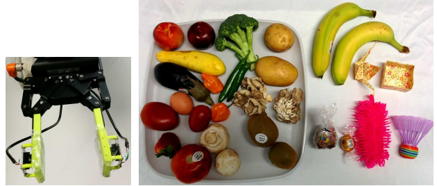
Fig.1 Left: Robotiq gripper with FingerVision sensors. Right: 30 objects used in the experiment.
