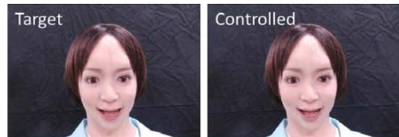
**Fig.6** Image comparison of the resulting face when the solver output are applied to the android for the case of target feature points captured from random actuator displacements.
